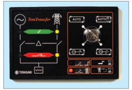
The controller features a self seeking power supply which will utilise power from the Mains AC supply or the Generator AC supply. A DC supply to the module is not essential for basic operation, though some 'higher' functions require it (such as system diagnostics).
